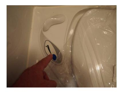
The toilet comes with chemicals that can be poured into the cassette unit from <u>outside</u>. **Do not** add the chemicals from inside the toilet to the flush water, as they will damage the seals in the toilet. Always add chemicals to the cassette on the outside of the unit.
